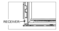
If receiver removal is necessary, remove the left access panel from the front of the appliance. Remove the 2 screws holding the receiver in place. Pull the receiver through the access hole and replace.
